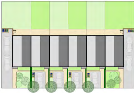
Side parking at end of terrace with single parking to front.
